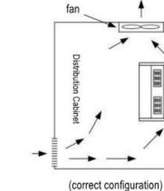
${}^{\bullet}\!Please$  position the inverter front forward and top up for heat dissipation.
